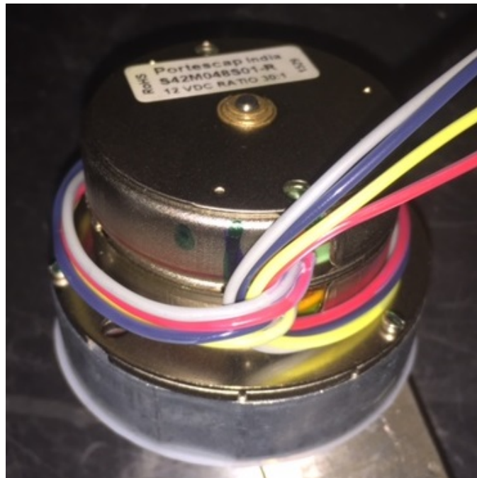
Figure 5 – IGV Motor Wiring
