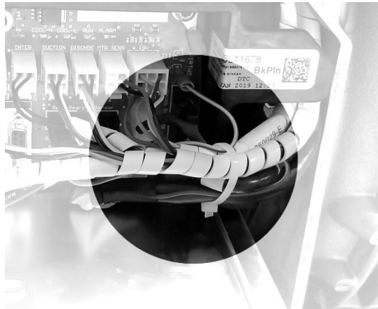
Figure 20 – Backplane Harness Cable Tie
