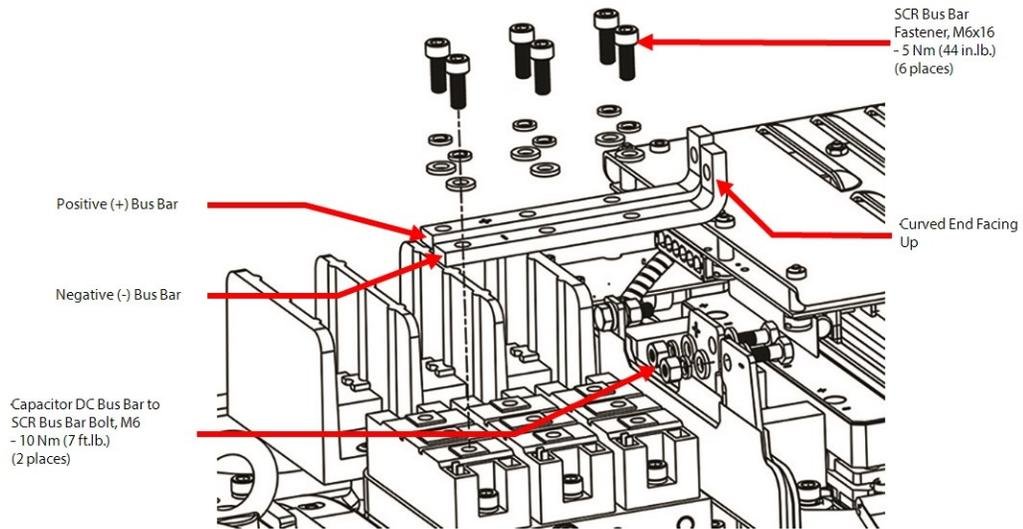
9. Remove the two (2) M6x16 fasteners that secure each SCR to the SCR Cooling Manifold and remove the SCRs. Refer to Figure 4-155 SCR Removal - TTS300/TGS230 for this and the following step.
