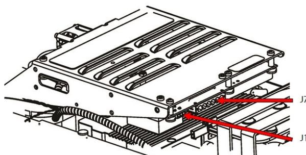
2. Connect the two (2) plugs of the compressor cable harness into the corresponding sockets of the DC bus test harness. Refer to Figure 1-14 Connect DC Bus Test Harness (Closed-Top Soft Start) for this and the following step.
