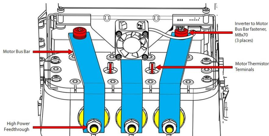
12. Install the Motor Bus Bars. Refer to Section 4.23.5 Motor Components Removal and Installation on page 196.
