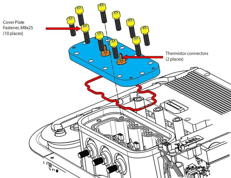
6. Remove the 10 M8x25 fasteners that secure the Cover Plate to the Main housing. Refer to Figure 4-222 Motor Cover Plate Removal.
