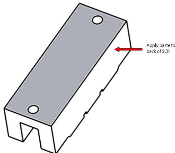
4. Install the SCRs on the SCR Cooling Manifold. The SCR Gate Connectors should be on the same side as the Discharge P/T Sensor. Refer to Figure 4-163 SCR Orientation - TTS300/TGS230 on page 154 for this and the following step.
