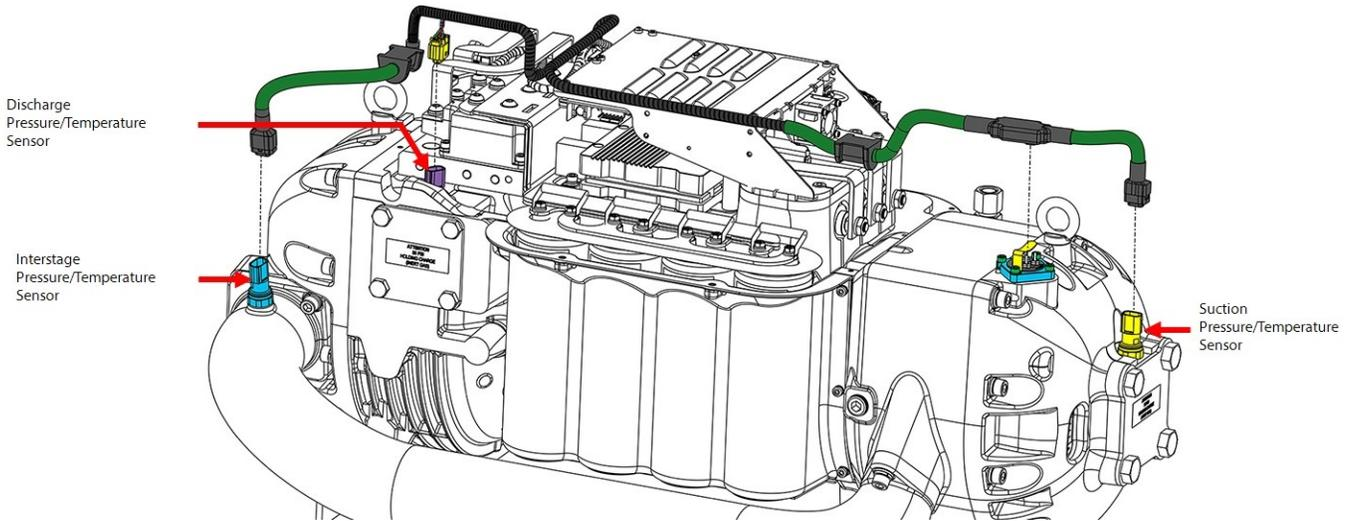
The sensor connector clips link to the compressor control cable which then connect to the Backplane at J18 and J19 (and J17 for TTH/TGH only).
