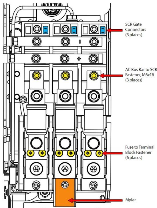
6. Remove the bolts that secure the (+) and (-) SCR Bus Bars to the DC Bus Bars. Refer to Figure 4-154 DC Bus Bar Removal - TTS300/TGS230 on page 150 and Figure 4-155 SCR Removal - TTS300/TGS230 on page 150 for this and the following two (2) steps.
