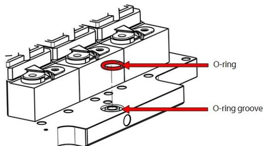
3. Clean the O-ring grooves in the SCR Manifold Return Brass Fitting with a lint-free cloth.
