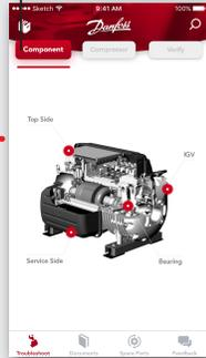
The user can select from a list of symptoms in the app that match the problems exhibited by the compressor being serviced. The app will then list potential causes, solutions to the problem, and service literature to reference for further information.
