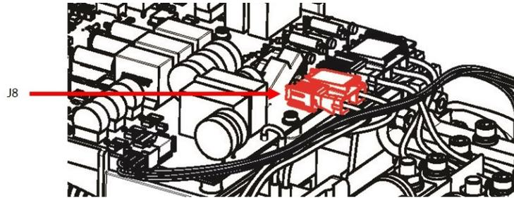
2. Connect the plug of the compressor cable harness into the corresponding socket of the DC bus test harness. Refer to Figure 1-18 Connect DC Bus Test Harness (Open-Top Soft Start) and Figure 1-19 DC Bus Test Harness Connection Diagram (Open-Top Soft Start) for this and the following step.
