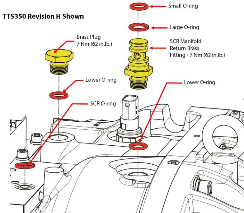
5. Carefully install the SCR Cooling Manifold over the SCR Manifold Return Brass Fitting. Press down firmly to ensure proper seating of the O-rings into the plate.
