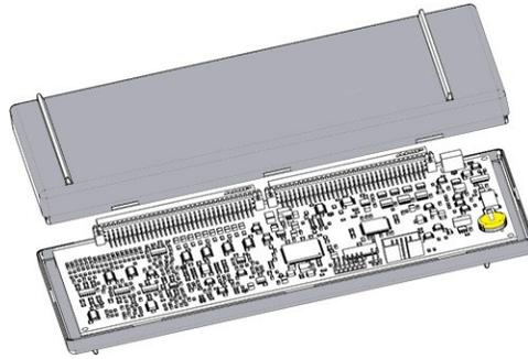
3. Set the multimeter for voltage measurements and place the red (+) probe on the battery itself (top) and the black (-) probe on the ground terminal shown below.
