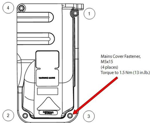
3. Follow the sequence twice. The first time, only tighten the fasteners halfway down to allow for adjustment. Tighten the # 4 fastener only once and be sure to not overtighten. Torque to 13 in.lb. on the second pass.
