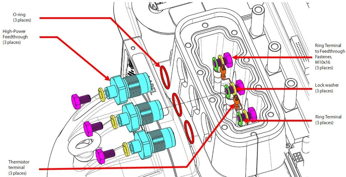
8. Remove the three (3) M10 nuts, lock washers, and ring terminal connections from the feedthrough in order to be able to release feedthrough assembly. Refer to Figure 4-226 High-Power Feedthrough Removal (stainless steel).
