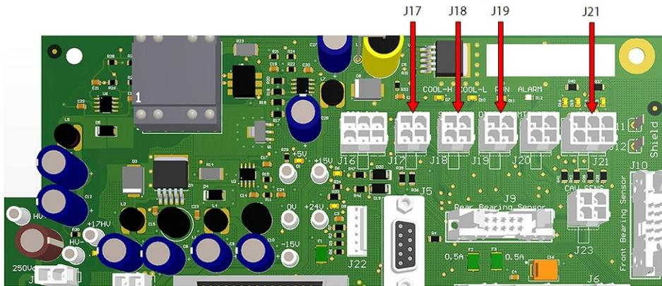
7. Disconnect the cables from the suction and discharge pressure sensors. Refer to Figure 4-23 Pressure/Temperature and SCR Temperature Sensor Locations - TTS300/TGS230 on page 69, Figure 4-24 Pressure/Temp and SCR Temp Sensor Locations - TTS/TGS (Except TTS300/TGS230) on page 69, and Figure 4-25 Pressure/Temperature Sensor Locations - TTH375/TGH285 on page 69 for this and the following step.
