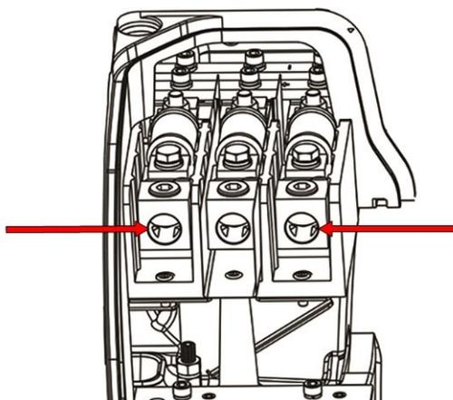
**Figure 4-80 Measuring 3-Phase AC Input Voltage on AC Input Terminals (TTS/TGS/TTH/TGH (Except TTS300/TGS230))**
