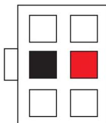
6. Reverse the multimeter leads on the 24VDC output terminals and measure the resistance. The result should be a rising or falling value, not static, zero, or infinity.
