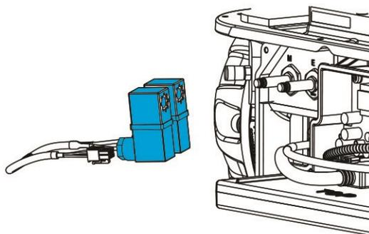
7. Remove any debris or dust from Backplane Board and solenoids using a soft-bristle brush.
