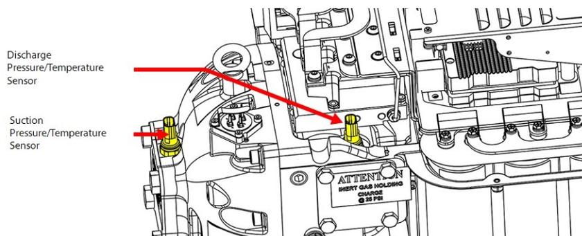
**Figure 4-272 Pressure/Temperature Sensor Locations (TTH/TGH)**
