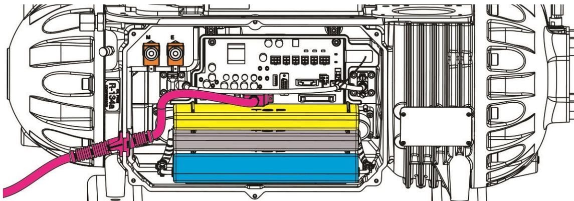
5. Remove the Motor-Cooling Valve Solenoid Coils by removing the retaining nut on each solenoid.
