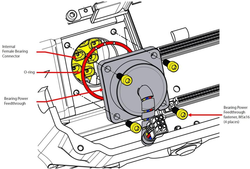
9. Remove the Feedthrough.
