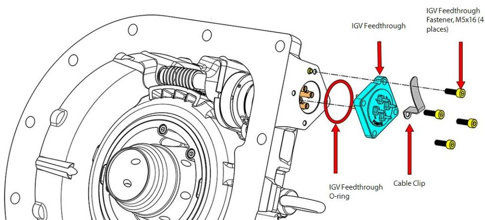
3. Disconnect the four (4) wires from the four-pin Feedthrough. Note and record position of wire colors to their corresponding pins. Expected: 1 = Red, 2 = Gray, 3 = Yellow, and 4 = Black. Refer to Table 4-15 IGV Feedthrough Wiring Order on page 92.
