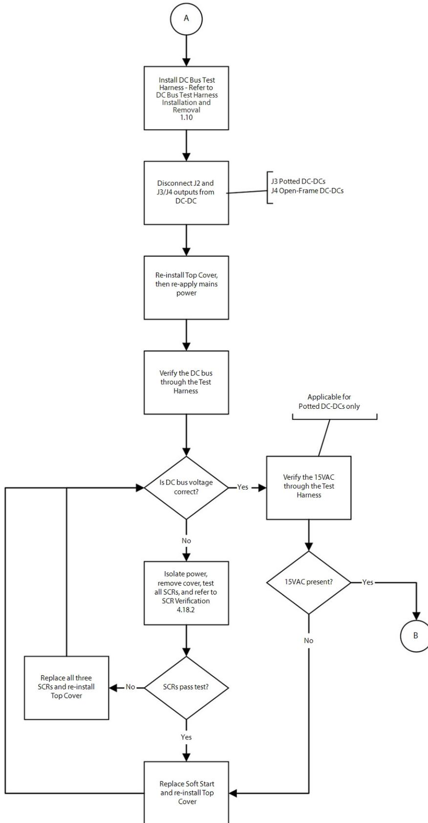
Figure B-5 Compressor Voltage Troubleshooting Flowchart (Sheet 3)
