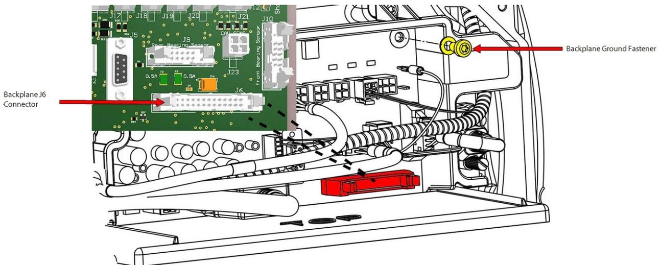
9. Cut any cable ties securing the Inverter Cable Harness and pull through the compressor housing passage.
