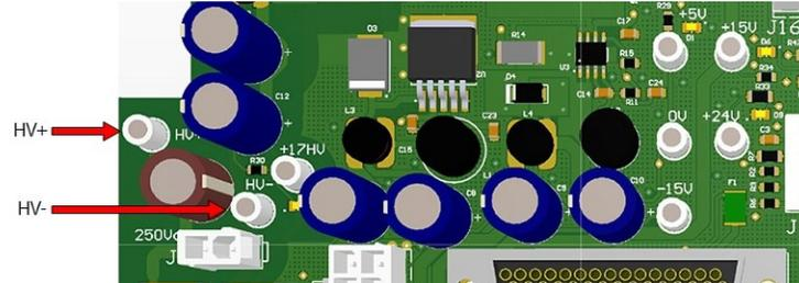
8. Still set on diode measurement, place the black (-) multimeter lead on the HV+ test point of the Backplane and the red (+) multimeter lead in the first pin hole of the PWM connector, ensure the lead makes contact with the clip in the pin hole. Refer to Figure 4-253 Connecting Leads to PWM Connector and HV- and HV+ Test Points. The measured voltage drop should be 0.39-0.46VDC.
