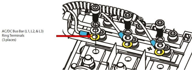
3. Disconnect the two (2) -DC ring terminals from the -DC bus bar by removing the attaching hardware. Refer to Figure 4-129 DC Ring Terminal Removal - TTS300/TGS230 for this and the following step.
