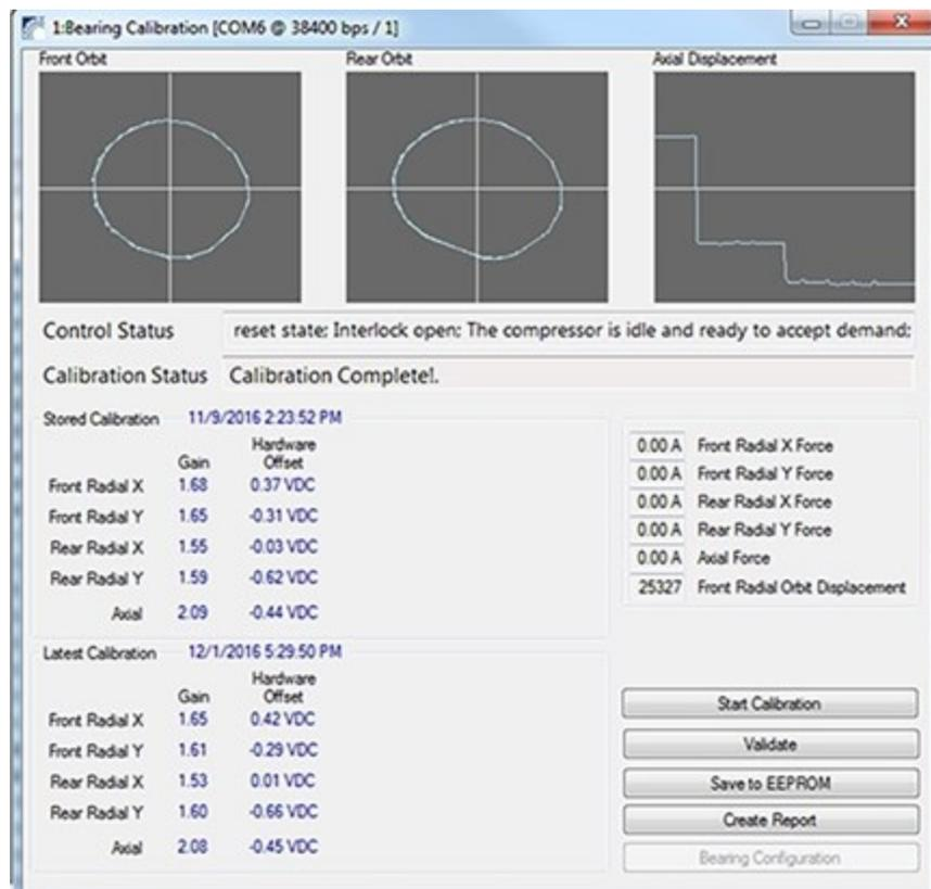
If the message “Calibration Failed” or “Levitation Failed” appears when attempting to calibrate, it indicates the steps expected by the SMT have not been completed. To determine the cause of failure, verify the following:
