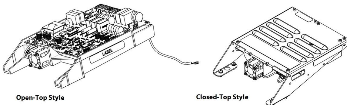
The Soft Start limits in-rush current when power is applied to the compressor by progressively increasing the conduction angle of the voltage through the SCRs to charge the DC capacitors. It uses a 3-phase voltage input at 50/60Hz, between 380-575VAC, and a DC voltage signal from the SCR output to generate output pulses of 0-12VDC to the SCR gates for the in-rush current control signal.
