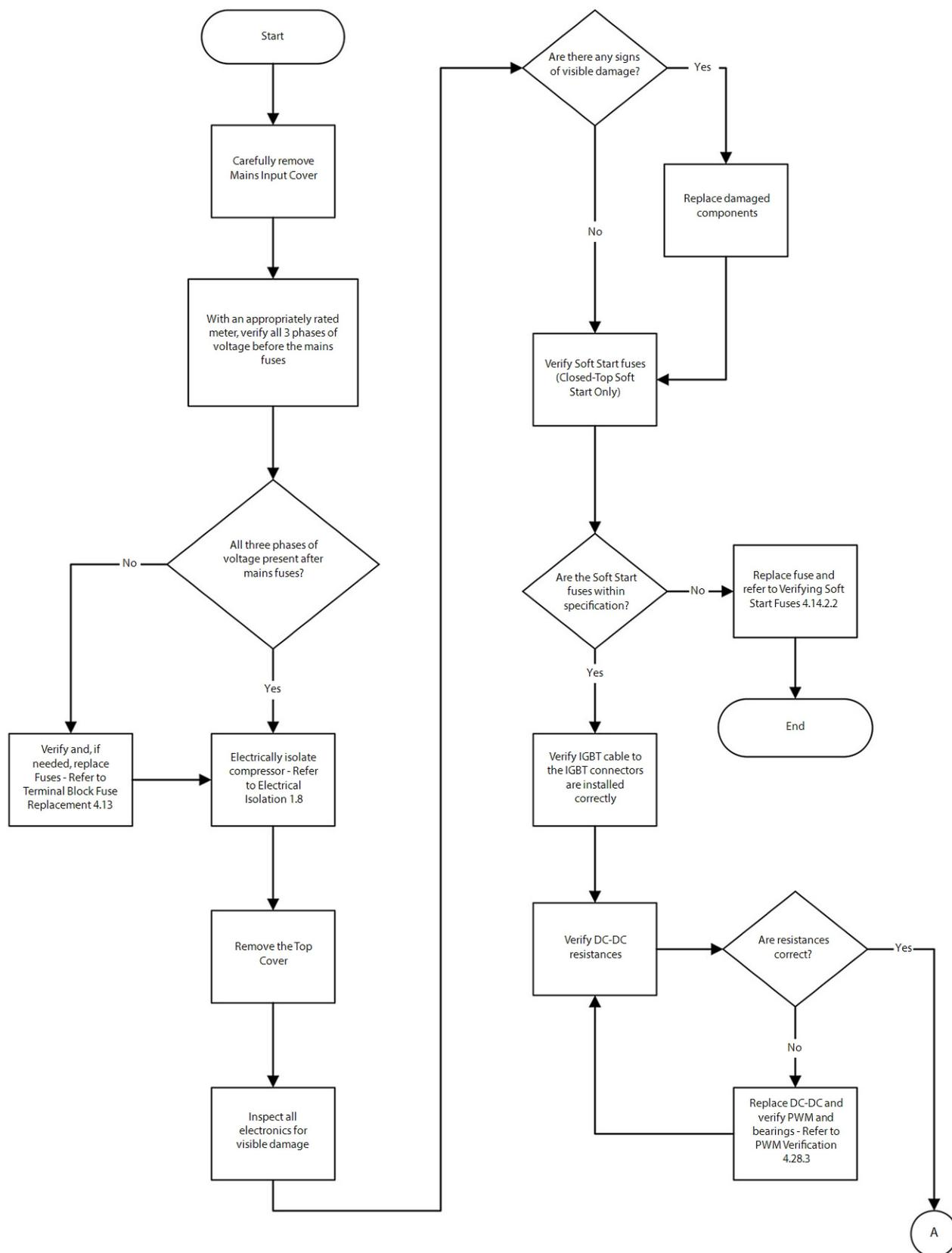
Figure B-4 Compressor Voltage Troubleshooting Flowchart (Sheet 2)
