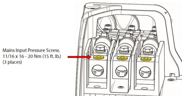
**Figure 4-75 Mains Input Nut Installation - TTS/TGS/TTH/TGH (Except TTS300/TGS230)**
