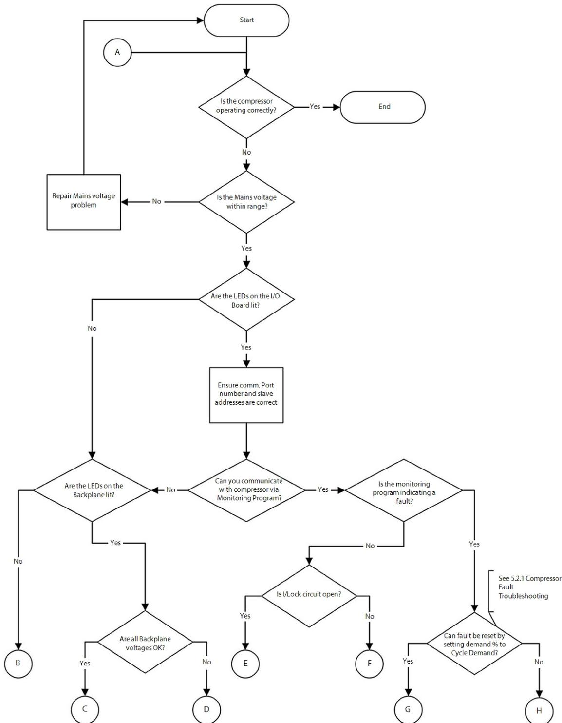
Figure B-2 Compressor Operation Troubleshooting Flowchart (Sheet 2)
