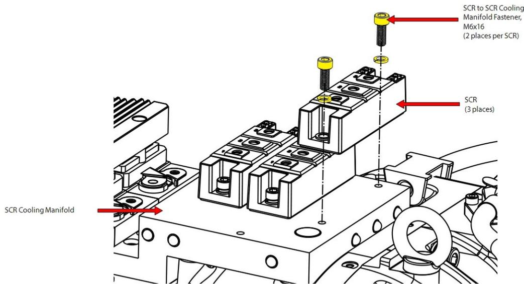
8. Clean the heat sink paste from the SCR and Manifold using a cloth and isopropyl Alcohol.
