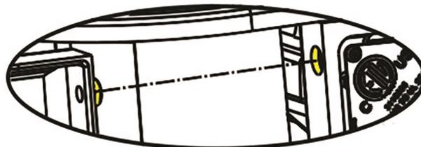
5. Place the long M5x20 fastener and flat washer in position number three (3) shown in Figure 4-15 Capacitor Cover Torque Sequence. Use the remaining M5x15 fasteners to secure the cover. Tighten all fasteners according to the sequence in Figure 4-15 Capacitor Cover Torque Sequence. Torque to 13 in.lb. on the second pass.
