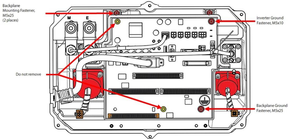
10. Remove the Backplane Frame from the compressor housing.
