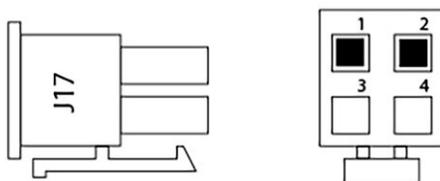
4. Using a multimeter set for resistance measurements, place the leads in terminal 1 and 2 of the cable plug. Refer to Figure 4-146 J17 Connector. The value should correspond with a negative temperature coefficient (NTC) thermistor 10K $\Omega$  @ 70°F (21° C). Refer to Figure 4-273 Temperature vs. Resistance on page 246.
