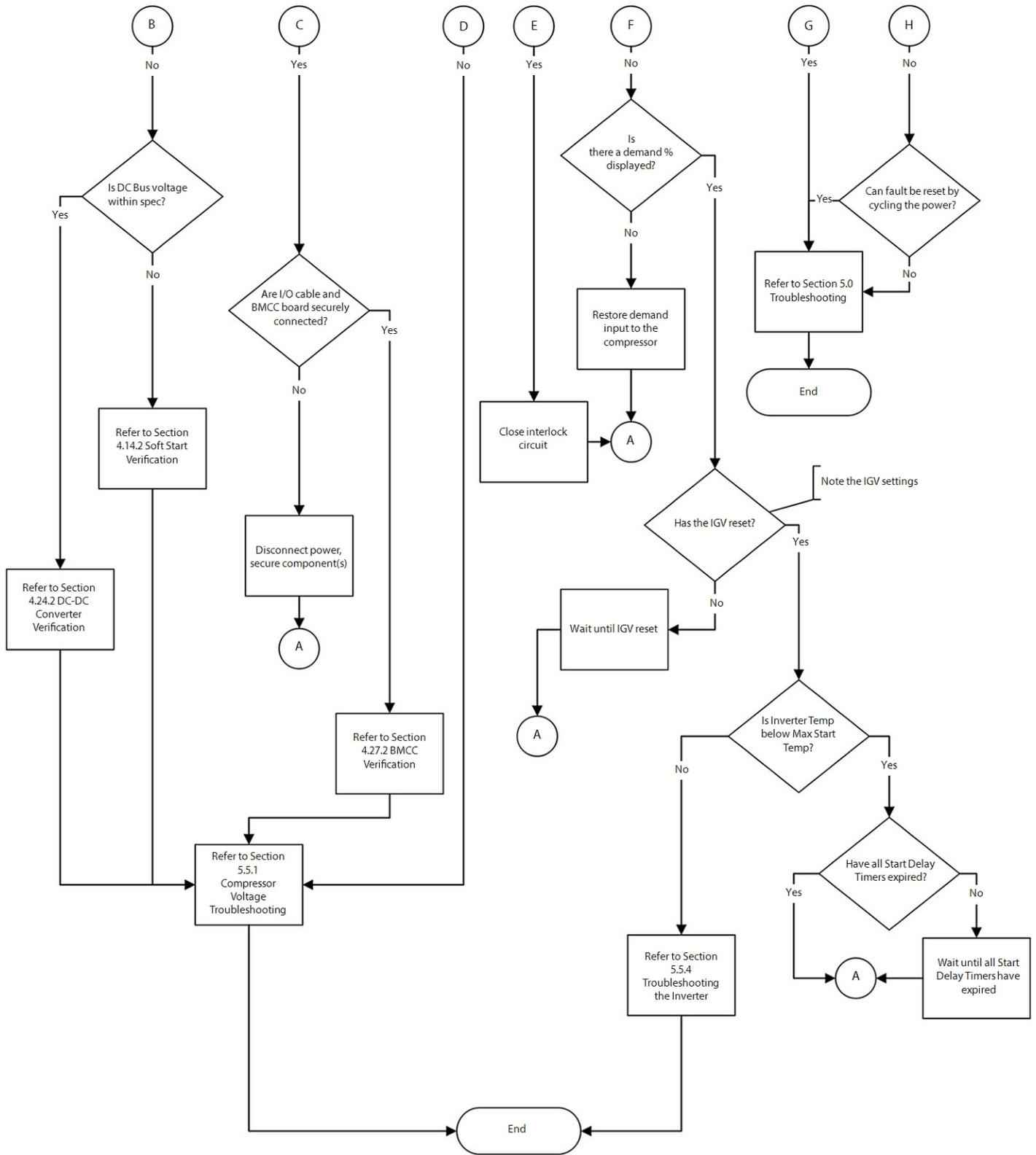
Figure B-3 Compressor Voltage Troubleshooting Flowchart (Sheet 1)
