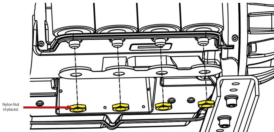
5. Carefully lift the DC Bus Bars and capacitors out as an assembly. Do not remove the bleed resistors or capacitors from the bus bars. Refer to Figure 4-182 Capacitor Assembly Removal - TTS300/TGS230 on page 170.
