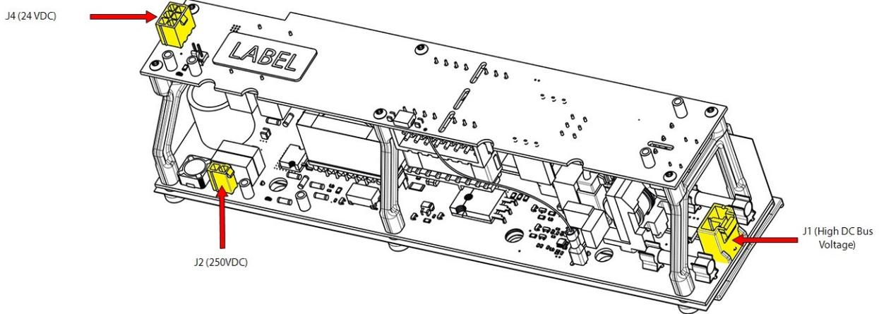
4. Loosen the M3x10 fasteners that are located next to the Inverter. Refer to Figure 4-231 DC-DC Converter Removal on page 207 for this and the next two (2) steps.
