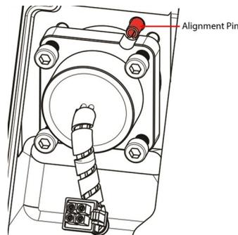
5. Finger-tighten the four (4) M5x16 fasteners and then torque in a crisscross pattern to 3 Nm (27 in. lb.) and then to a final torque of 5 Nm (44 in.lb.). Refer to Figure 4-261 Bearing Power Feedthrough Torque Sequence.
