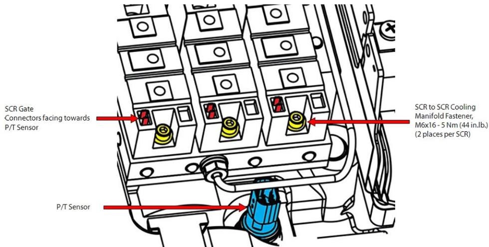
6. Place the negative bus bar on the SCRs. The negative bus bar should be next to the SCR Gate Connectors (aligned with the holes identified as #3 on the SCRs). Refer to Figure 4-164 Bus Bar Installation - TTS300/TGS230 and Figure 4-165 Bus Bar Locations - TTS300/TGS230 on page 155.
