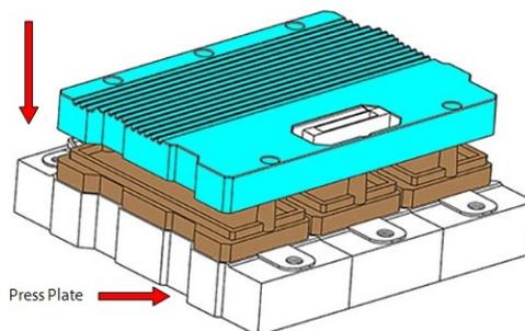
10. Insert the remaining fasteners and tighten from center outward according to Figure 4-216 Initial Tightening Pass Sequence on page 192. This will be the first pass and the fasteners should only be snug and not torqued at this step.
