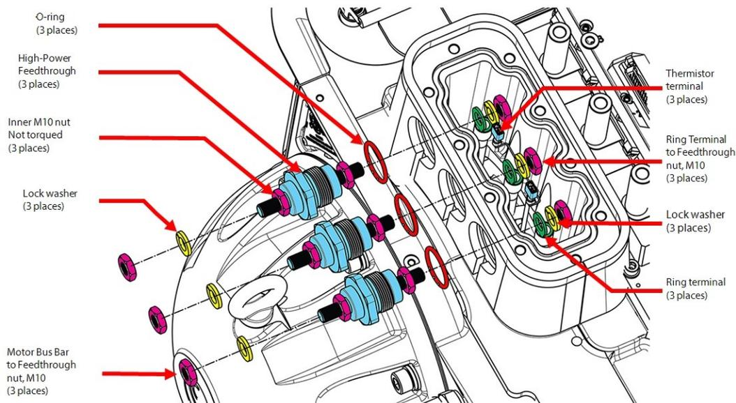
9. Remove the three (3) high-power feedthroughs using a 36mm wrench.
